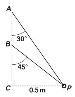
A small smooth ring *P* of mass 0.4 kg is threaded onto a light inextensible string fixed at *A* and *B* as shown in the diagram above, with *A* vertically above *B*. The string is inclined to the vertical at angles of 30° and 45° at *A* and *B* respectively. *P* moves in a horizontal circle of radius 0.5 m about a point *C* vertically below *B*.
